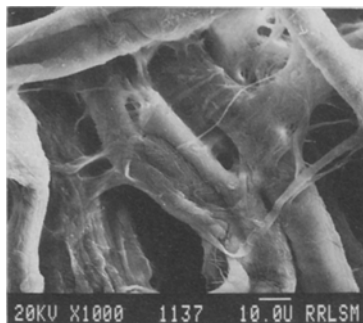
Fig. 5: SEM photo of \text{BF}_3 \cdot \text{OEt}_2 treated paper
