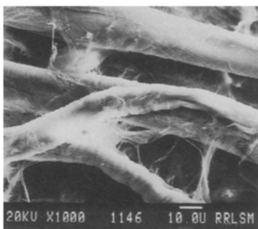
Fig.4: SEM photo of untreated paper
