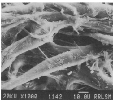
Fig. 6: SEM photo of grafted paper 1 hour reaction
